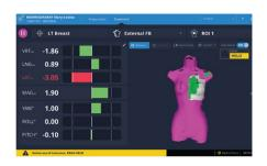
Users can create customized tolerance thresholds of movement; the radiation beam is automatically held\* if the patient moves out of tolerance.
