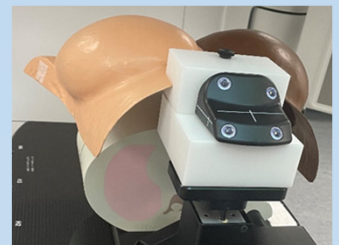
Figure 1: XENA phantom attached to the CIRS dynamic respiratory phantom with the Varian RPM block
